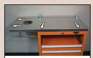
10. Set COUNTERTOP onto MAIN FRAME. Press down firmly to COMPLETELY FLATTEN silicone. Slide COUNTERTOP FULLY FORWARD and to the LEFT. Use masking tape to hold COUNTERTOP to side and back of tool chest while silicone dries.
