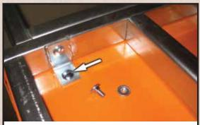
3. Drill 5/16" (8mm) holes at four marked locations. Attach MAIN FRAME to top of chest with SHORT CARRIAGE BOLTS (a) and NUTS (d). Tighten NUTS inside tool chest.
