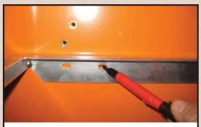
7. On LOWER SIDE FRAME, mark two hole locations that avoid reinforcements inside tool chest wall. Example: For Viper tool chest, mark the two inner holes in bracket.
