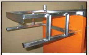
5. Attach all four CONNECTOR BRACK-ETS (I) to UPPER and LOWER SIDE FRAMES with PHILLIPS SCREWS (h). Position CONNECTOR BRACKETS with ribs facing out and long slots down. Gently tighten SCREWS.
