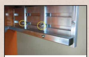
22. Mount SIDE COVERS onto ALUMINUM NUTS. Align SLATWALL SIDE COVERS parallel with outside lip of COUNTERTOP and tighten four PHILLIPS SCREWS.
