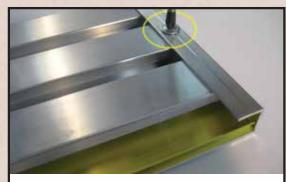
20. Attach SHORT SIDE MOLDINGS (J) to SLATWALL SIDE COVERS (K). Install one DRILL POINT SCREW on back of each molding. Highlighted yellow area in photo indicates back of SLATWALL SIDE COVER.
