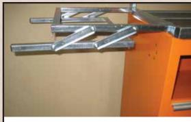
8. Rotate LOWER SIDE FRAME up. Drill two marked holes with 5/16" drill. Rotate LOWER SIDE FRAME down. Fasten LOWER SIDE FRAME with PHILLIPS SCREWS (f) and NUTS (d). Tighten NUTS inside tool chest. Tighten CONNECTOR BRACKET SCREWS.
