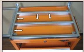
2. Place MAIN FRAME (A) on top of tool chest. Push FRAME against the LEFT and BACK lip of tool chest. Mark the location of four square mounting holes on top of tool chest. Remove MAIN FRAME.
