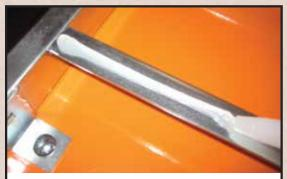
9. Apply a 1/8" bead of pure silicone from a caulking gun onto top surfaces of MAIN FRAME and UPPER SIDE FRAME. Dab some silicone around carriage bolt heads to ease disassembly if needed.
