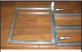
1. Connect UPPER SIDE FRAME (G) to MAIN FRAME (A) with LONG CARRIAGE BOLTS (g) and FLANGE NUTS (d). Insert BOLTS from right to left. Hand tighten NUTS.
