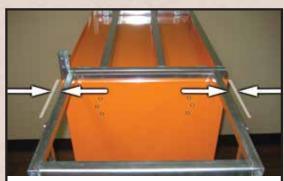
4. Tap UPPER SIDE FRAME (G) to a centered position on side of tool chest. Tighten NUTS (d) connecting UPPER SIDE FRAME to MAIN FRAME.
